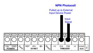
Figure 57 - NPN External Trigger Using External Power
