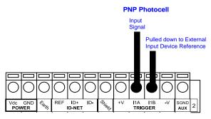
Figure 56 - PNP External Trigger Using External Power
