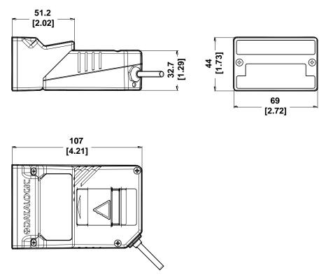
Figure 31 – Scanner + OM2000N Overall Dimensions
