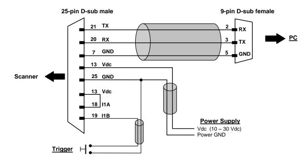
Figure 91- Test Cable for Serial Model Scanners
