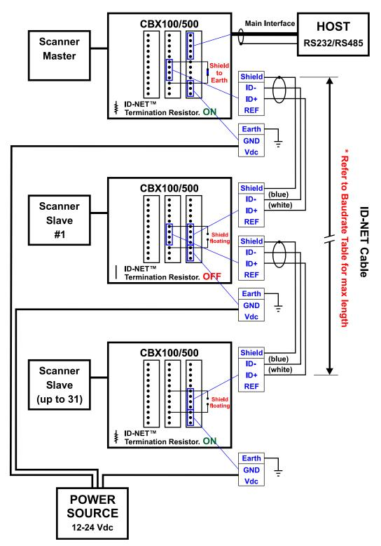
Figure 51 – ID-NET™ Network Connections with Common Power Star Network
