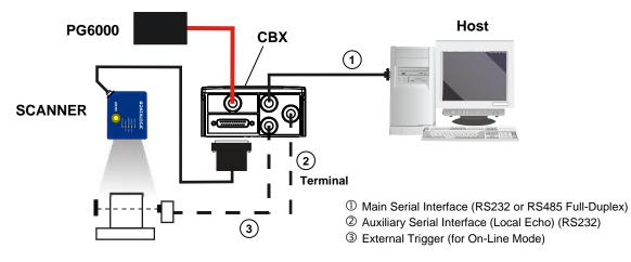
Figure 66 – Serial Interface Point-to-Point Layout
