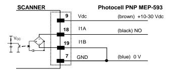
Figure 88 – MEP-593 PNP Photocell Connections Using Scanner Power
