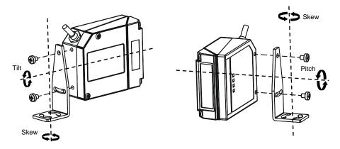
Figure 2 - Positioning with Mounting Bracket
