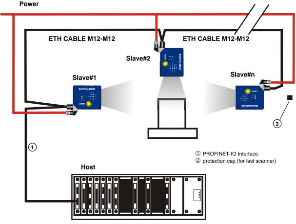
Figure 69 – PROFINET-IO Single Station Layout
