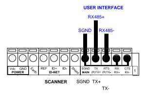
Figure 45 - RS485 Full-duplex Connections using Only TX Signals
