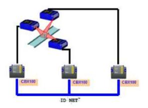
ID-NET<sup>™</sup> interface allows local connection of multiple scanners reading different sides of the same target. All scanners share a single presence sensor and activate/deactivate simultaneously.
