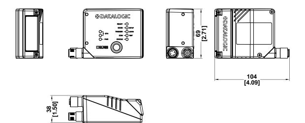
Figure 13 – x3xx Models Overall Dimensions with Connectors at 0°
