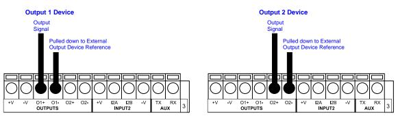
Figure 65 - NPN/Output Open Collector Using External Power
