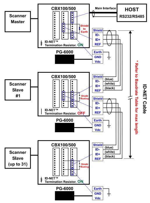
Figure 49 – ID-NET™ Network Connections with isolated power blocks
