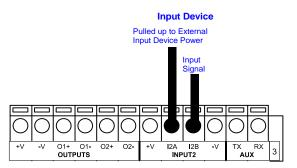
Figure 61 - NPN Input 2 Using External Power
