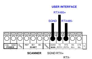
Figure 46 - RS485 Half-duplex Connections
