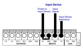
Figure 59 - PNP Input 2 Using Scanner Power
