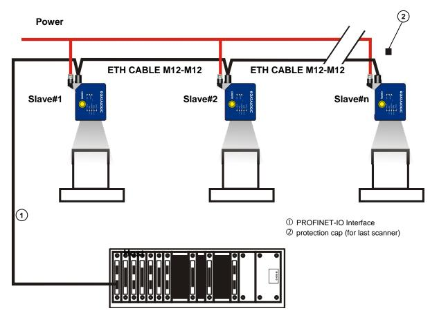
Figure 70 – PROFINET-IO Multi Station Layout
