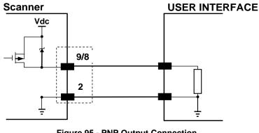
Figure 95 - PNP Output Connection
