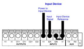
Figure 58 - PNP Input 2 Using Scanner Power
