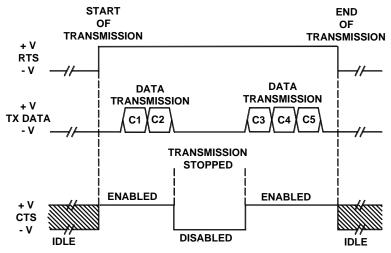
Figure 43 - RS232 Control Signals
