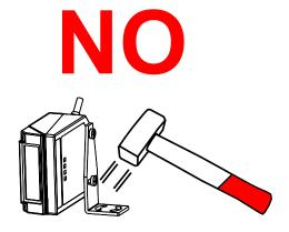
• do not weld the scanner into position which can cause electrostatic, heat or output window damage.
