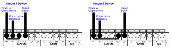
Figure 62 - PNP/Open Emitter Output Using Scanner Power
