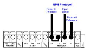
Figure 55 - NPN External Trigger Using Scanner Power
