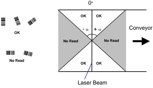
Figure 84 – Reading Zones with  $\alpha$  Max
