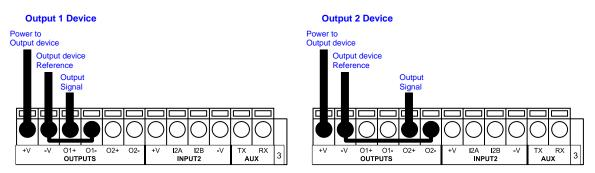
Figure 63 - NPN/Open Collector Output Using Scanner Power
