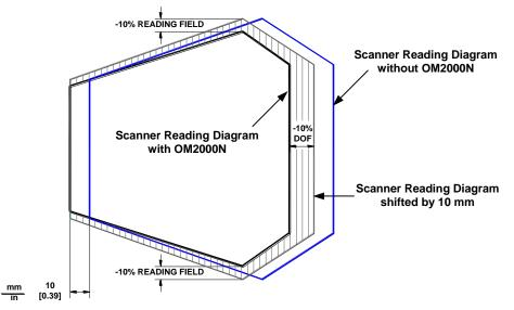
Figure 36 – OM2000N Reading Performance Comparison
