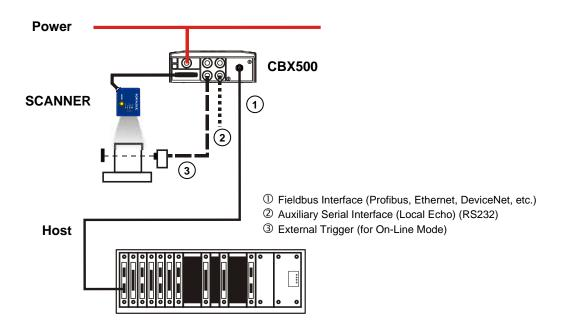
Figure 67 – Fieldbus Interface Point-to-Point Layout
