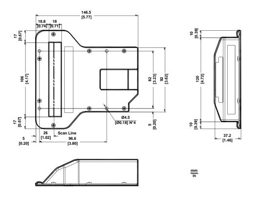
Figure 27 - GFC-200 Overall Dimensions
