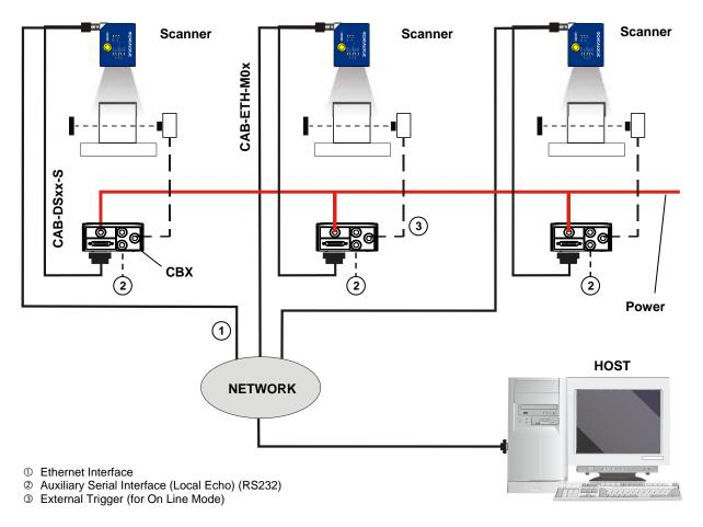
Figure 68 - Ethernet TCP/IP Network Layout
