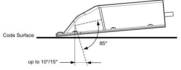
Figure 29 – Maintaining Minimum Skew Angle
