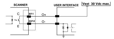
Figure 89 - Open Emitter Output Connections
