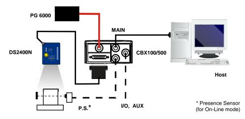
Figure 1 – Scanner in Stand Alone Layout
