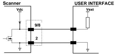
Figure 96 - NPN Output Connection
