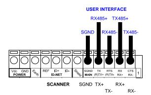
Figure 44 - RS485 Full-duplex Connections
