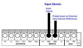
Figure 60 - PNP Input 2 Using External Power
