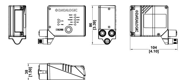
Figure 15 – x4xx Models Overall Dimensions with Connectors at 0°
