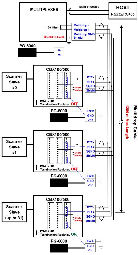
Figure 47 - Multidrop Connection to a Multiplexer
