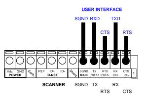
Figure 42 – RS232 Main Interface Connections Using Hardware Handshaking
