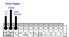
Figure 41 - Power Supply Connections
