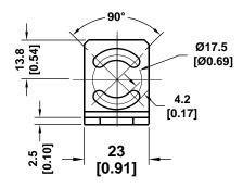
Figure 16 – Mounting Bracket Overall Dimensions
