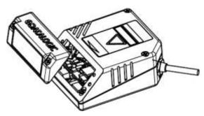
Figure 32 – Remove Scanning Window
