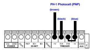
Figure 54 – PH-1 (PNP) External Trigger Using Scanner Power
