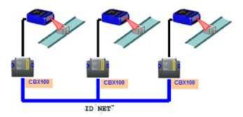
ID-NET<sup>™</sup> interface allows connection of scanners reading objects placed on independent conveyors. All scanners are typically located far away from each other and they use a dedicated presence sensor.
