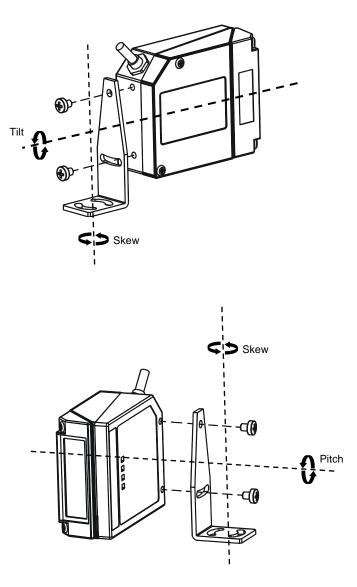
Figure 17 – Positioning with Mounting Bracket
