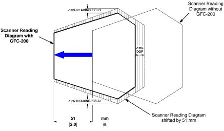
Figure 30 – GFC-200 Reading Performance Comparison
