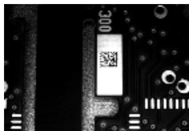
Figure 21 – Dot Matrix Code Directly Marked on PCB Copper Pad by Using Ink-Jet Technology
