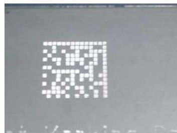
Figure 25 - Dot Peening Marking on Metal Surface with Multi-dot per Code Element
