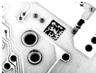
Figure 28 - Data Matrix Code Directly Marked on PCB Surface by Using Laser Etching Technology
