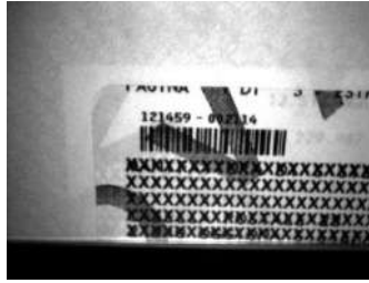
Figure 22 - Overprinted Barcode Readable by Matrix 410N also Through the Envelope Window Film
